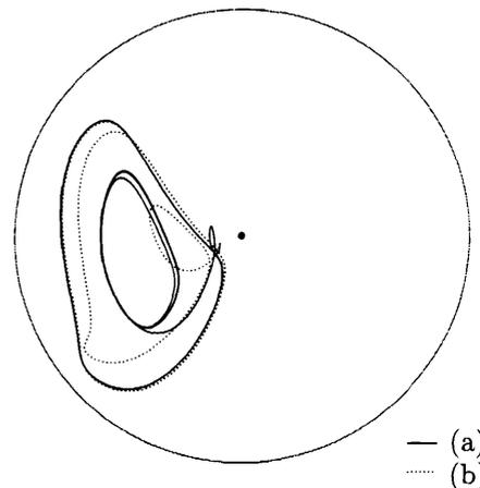
Figure 5: Comparison of the paths of (a) variable-film single-phase and (b)  $\pi$ -film double-phase cavitation models for a journal of  $M_e = 1.75 \times 10^4$  kg/m,  $\omega=350$ rad/s,  $(\epsilon_o, \phi_o)=(0.10, 0.35)$ ,  $F_p = 2 \times 10^5$  N/m,  $F_c=0$  N/m with time  $t \in [0, 0.15]$ .
