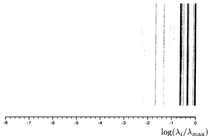
Figure 2: Eigenvalue spectrum of preconditioned system with  $P=B$  with  $(N, E_r, E_a) = (7, 2, 2)$  and illustration of model for the case of  $\alpha = 5.3 \times 10^{-2}$ ,  $\epsilon=0.5$ . The result is a condition number  $\kappa=188.3$  and number of PCG iterations = 28
