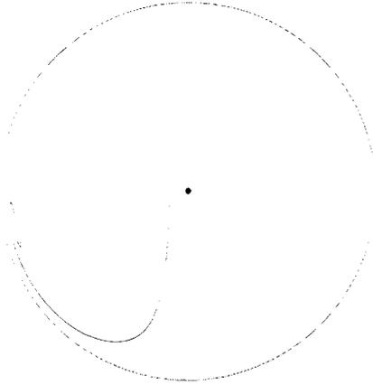
Figure 8: The path of journal with a full-film variable viscosity lubricant with  $M_e = 7 \times 10^4$  kg/m,  $\omega=250$ rad/s,  $(\epsilon_0, \phi_0)=(0.1, 0.0)$ ,  $F_p=F_c=0$  N/m with time  $t \in [0, 0.1]$ . The viscosity parameters are given in the paper.
