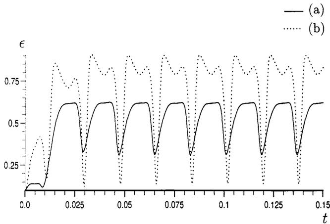
Figure 6: Plot of (a),(b) the eccentricity of the two journal paths shown in Figure 5a,b respectively.
