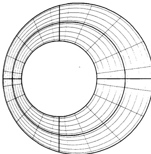
Figure 1: A spectral element discretisation of the journal bearing problem with  $E_a = 4$ ,  $E_r = 2$  and  $N = 7$ .
