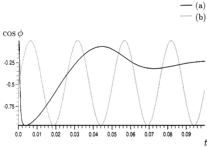
Figure 10: Plot of (a) the cosine of the attitude angle of the journals path shown in Figure 8 together with (b)  $k_1 + k_2 \sin(\omega t)$  for reference with the journal's angular velocity.
